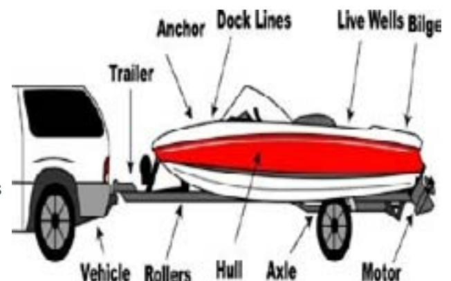
This Montana Fish, Wildlife & Parks illustration shows key areas to inspect, clean & dry on any boat. Make sure your watercraft & equipment is completely drained and dried. Questions? Contact FWP at (406) 444-2449.
