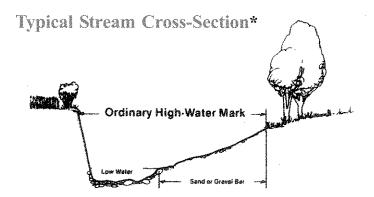
\* Although this is typical of some stream cross-sections, many other situations exist. Also, vegetation such as grass, sedges or willows can exist within the ordinary high-water marks. When in doubt, refer to the definition of ordinary high-water mark.
